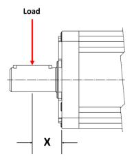
Figure 3-3 Radial Loading
