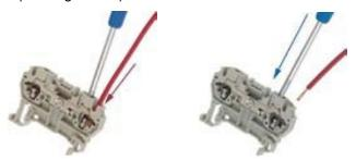
Figure 5-2 Screwdriver to Open the Terminal
