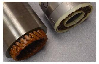
Figure 4: End turn length comparison
