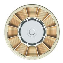
Figure 3: Minimized, non-overlapping end turns
