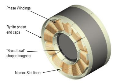
Thermally Conductive Epoxy Potting (not shown) Figure 5: Insulation System. UL Class 180 H
