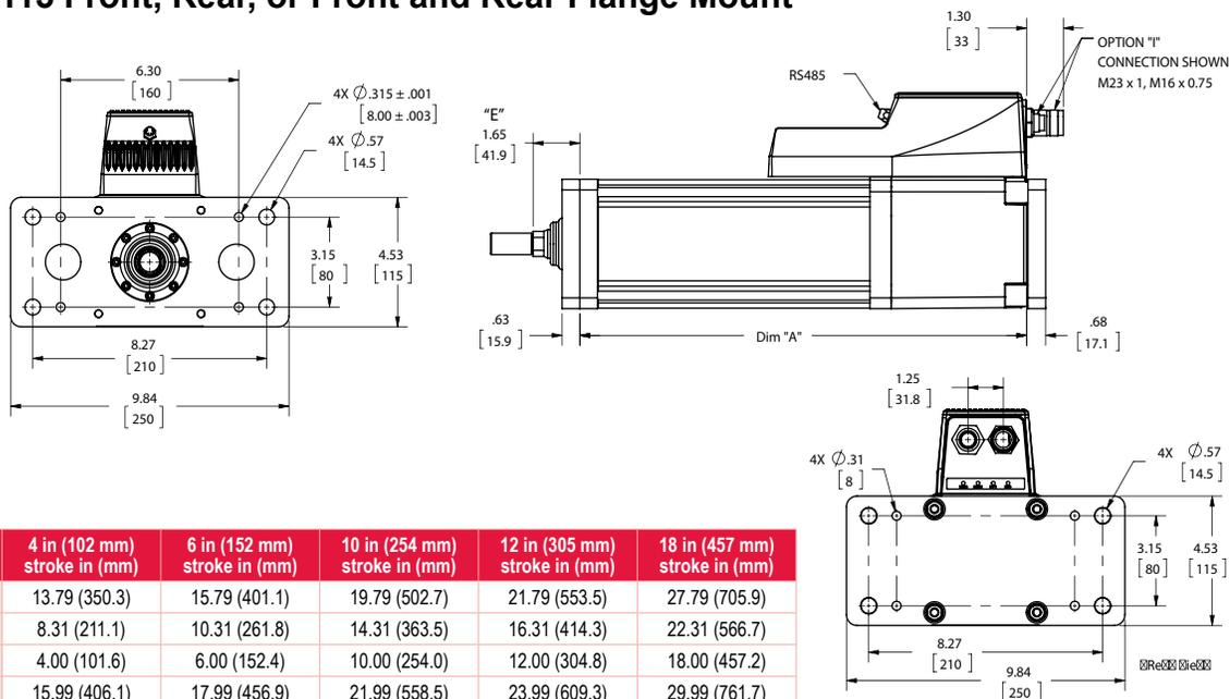
\* Add 2.33 inches to dimensions "A", "B" and "D" if ordering a brake. Add 1.77 inches to dimensions "A", "C" and "D" and dimension if ordering a splined main rod.
