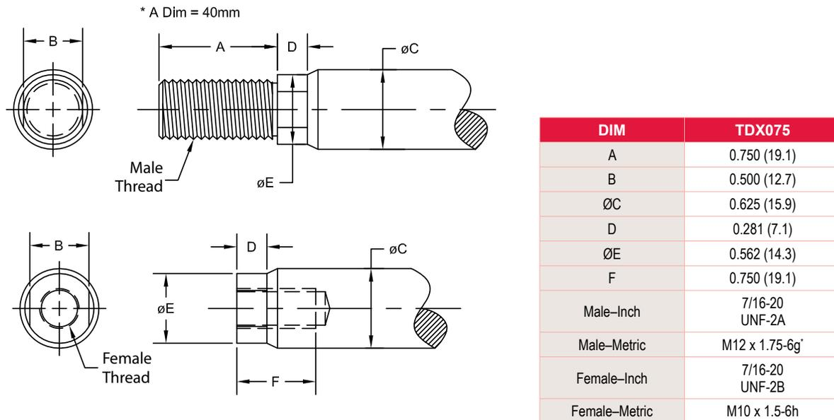
\*When ordering the male M12x1.75 main rod for the TDX075 dimension "A" will be 1.57 in (40 mm)
