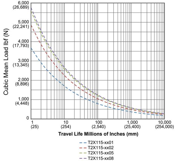
The L<sub>10</sub> expected life of a roller screw linear actuator is expressed as the linear travel distance that 90% of properly maintained roller screws are expected to meet or exceed. For higher than 90% reliability, the result should be multiplied by the following factors: 95% x 0.62; 96% x 0.53; 97% x 0.44; 98% x 0.33; 99% x 0.21. This is not a guarantee; these charts should be used for estimation purposes only.
