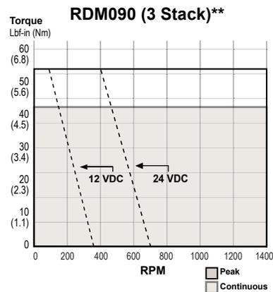
For RDG gearmotors, multiply torque by ratio and efficiency. Divide speed by gear ratio.
