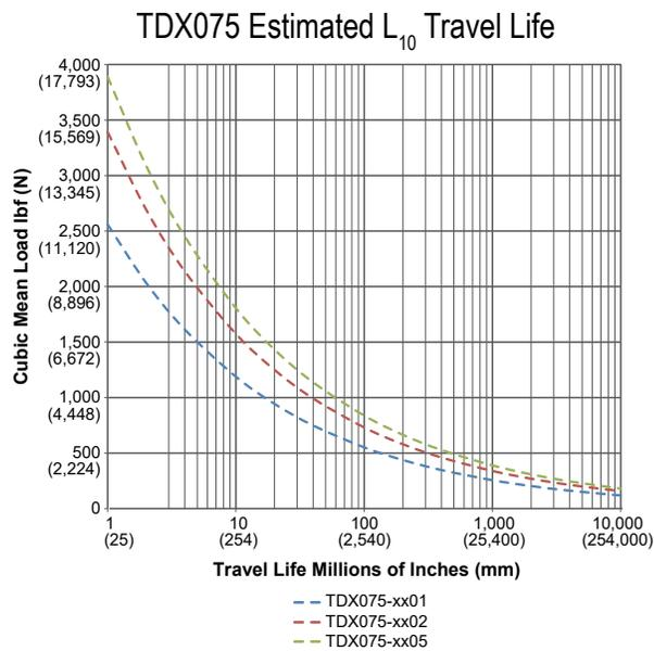
The L<sub>10</sub> expected life of a roller screw linear actuator is expressed as the linear travel distance that 90% of properly maintained roller screws are expected to meet or exceed. For higher than 90% reliability, the result should be multiplied by the following factors: 95% x 0.62; 96% x 0.53; 97% x 0.44; 98% x 0.33; 99% x 0.21. This is not a guarantee; these charts should be used for estimation purposes only.
