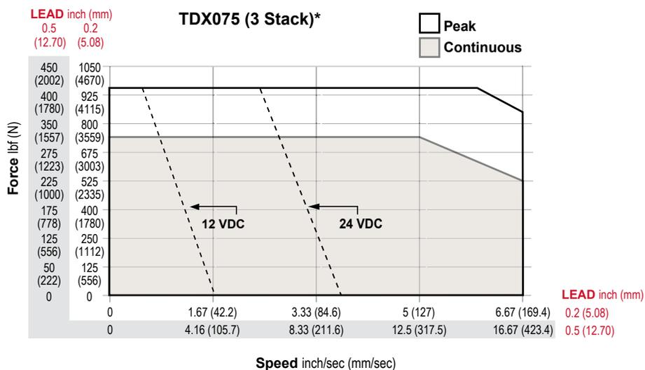
\*Test data derived using NEMA recommended aluminum heatsink 10" x 10" x 3/8" at 40°C ambient.
