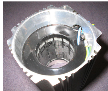
Figure 10 – T-LAM Stator Potted with Thermally Conductive Epoxy
